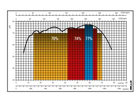
All the new Z6 series pumps offer a superior efficiency and therefore all points selected between 14 m<sup>3</sup>/h and 70 m<sup>3</sup>/h have always efficiency equal to or higher than 70% with a max efficiency of 77% within the overall Z6 range.
