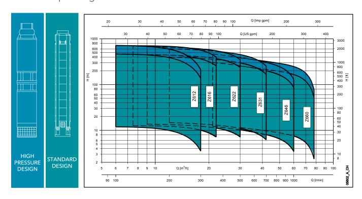
Z6 series operating characteristics at 60 hz.
